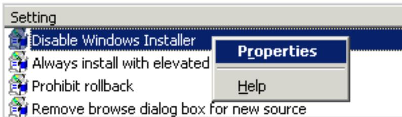
In the *Properties* window, select **Enabled** from the radio button options, and select **Never** in the *Disable Windows Installer*. Click **OK** when finished.
